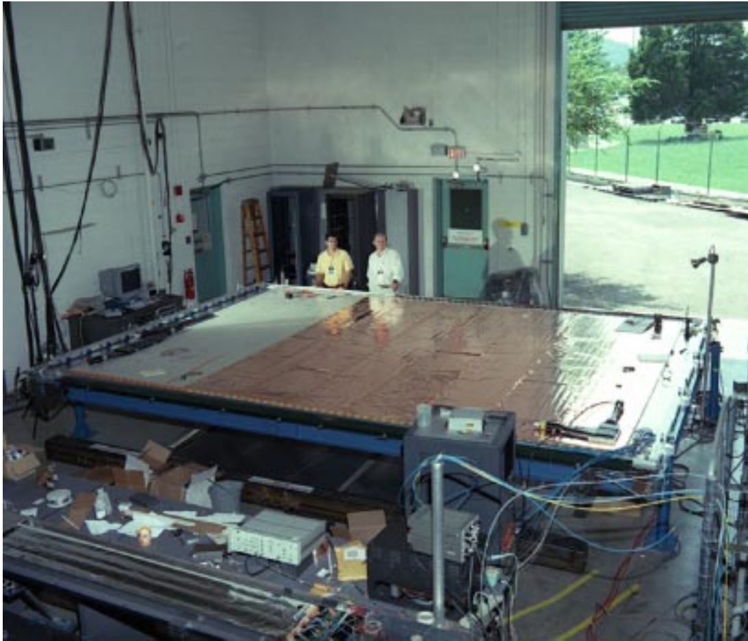
Figure 1: Full-scale prototype panel at ORNL. The streamer tubes (white) are mounted on the panel's aluminum midplane (tubes in the orthogonal orientation are on the underside of the midplane). The copper sheet serves as RF shielding and a capacitively coupled ground return path to terminate the anode signals.
